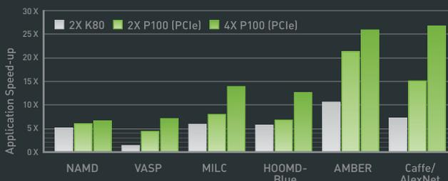
Dual CPU server, Intel E5-2698 v3 @ 2.3 GHz, 256 GB System Memory, Pre-Production Tesla P100
