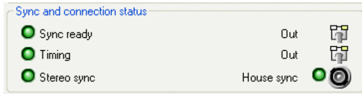
Figure 2.4 Sync and Connection Status for a Genlocked System
